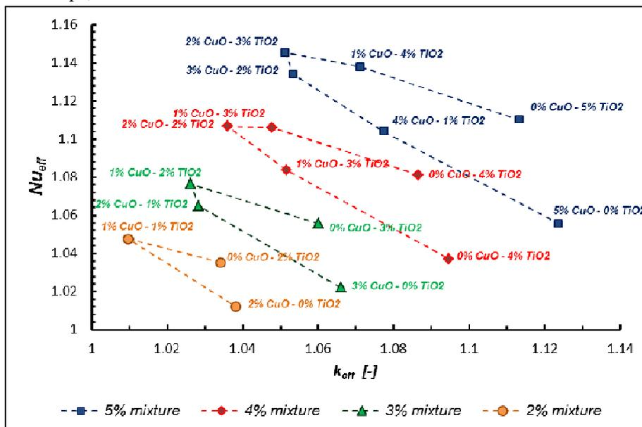
Figure 6. Distribution of average Nusselt number with respect to effective thermal conductivity for the hybrid nanofluid mixture for Reynolds number of 50,000
