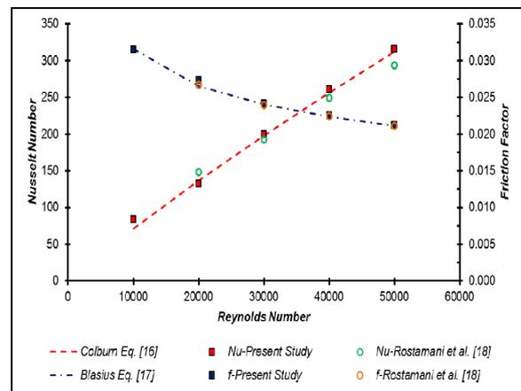
Figure 3. Comparison of distilled water results in terms of both Nusselt Number and friction factor as a function of Reynolds number
