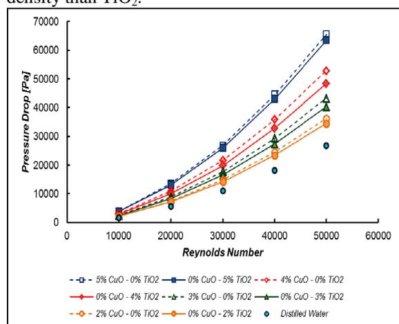
Figure 7. Volume fraction of used nanofluid mixture effect on pressure drop as a function of Reynolds number
