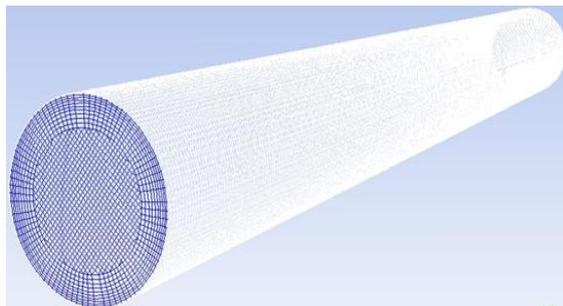
Figure 2. Grid structure of used circular tube
