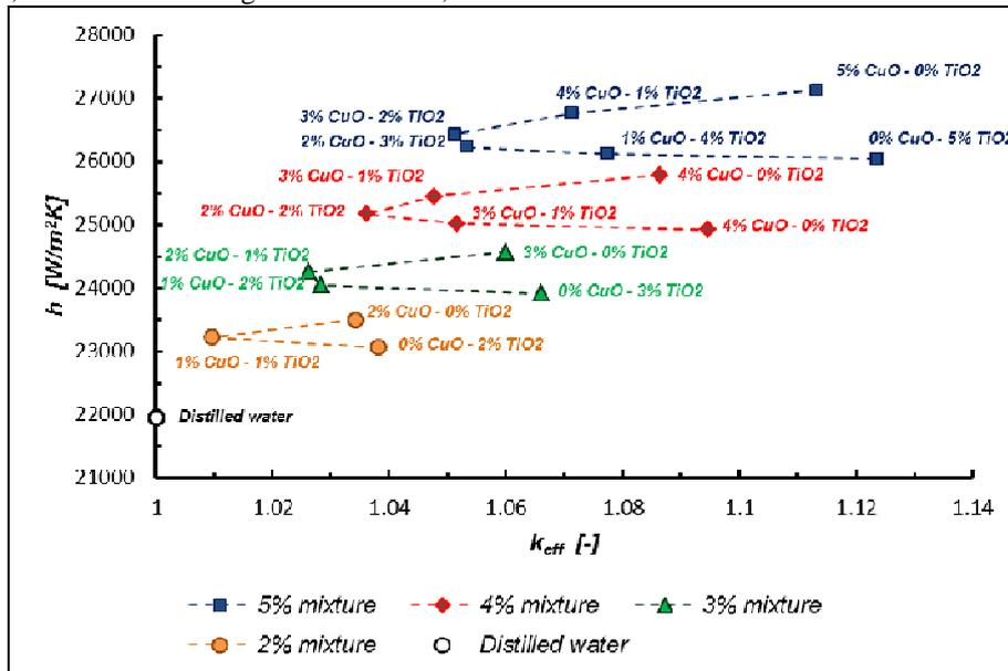
Figure 5. Convective heat transfer coefficient versus effective thermal conductivity for the hybrid nanofluid mixture
