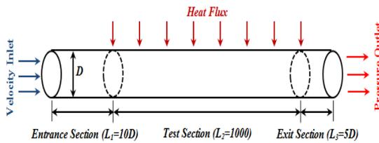
Figure 1. Schematic diagram of the computational domain
