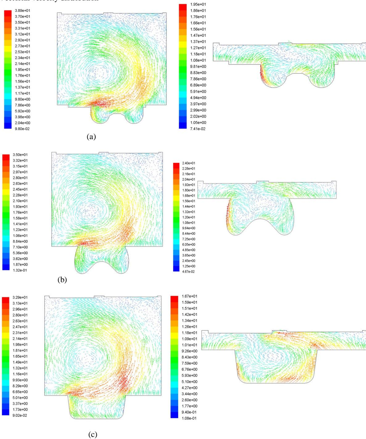
Fig.5 a, b, c: Velocity vectors at ABDC and TDC for three pistons
