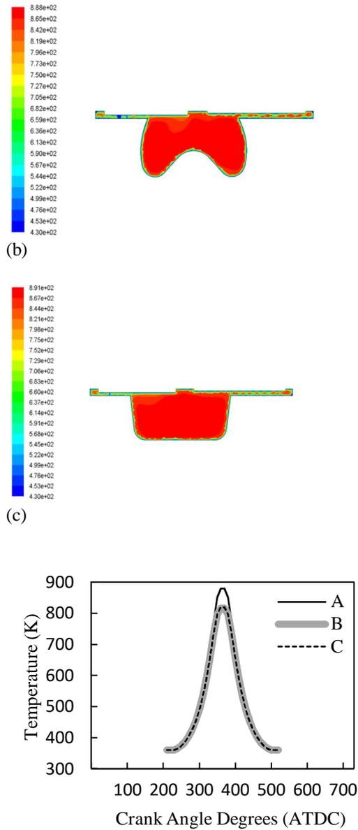
Fig: Calculated cylinder temperature versus crank angle compared for three pistons.
